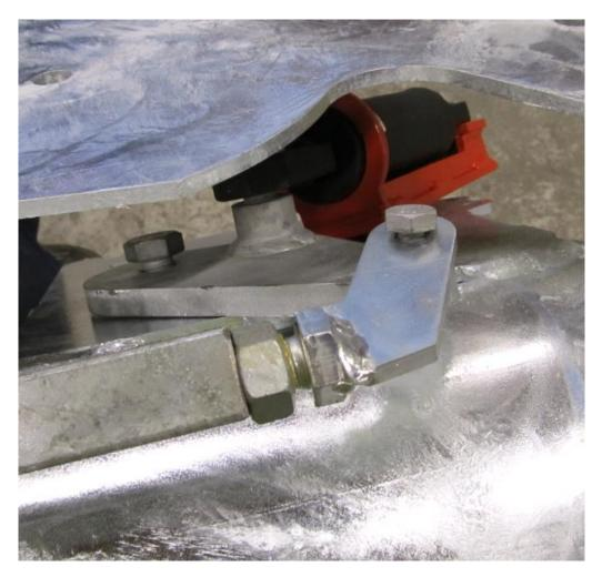
Tighten the screws that the parts could move. Apply grease to all moving joints and sliding surfaces.
