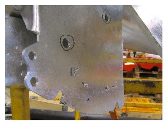
Attach the hydraulic unit in the marked holes as shown in the picture.
