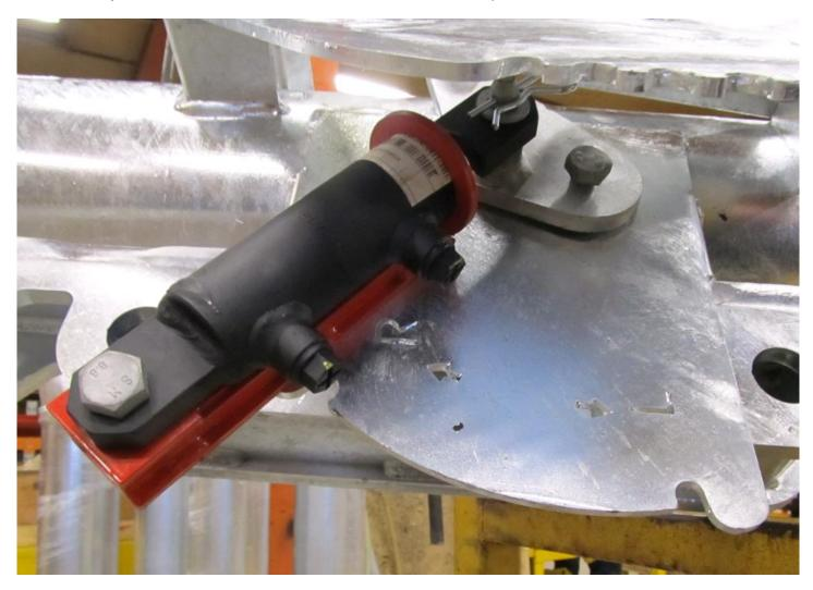
Attach to the rod for switching between loading/stirring.
